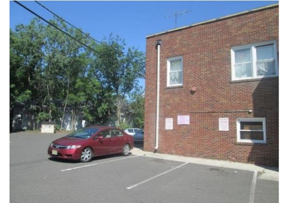
The rear of the shopping complex has a parking area which drains toward the street. Porous asphalt can be installed in the spaces along the building to infiltrate stormwater and capture roof runoff from the disconnected downspout. A preliminary soil assessment suggests that the existing soils have suitable drainage characteristics for green infrastructure.
