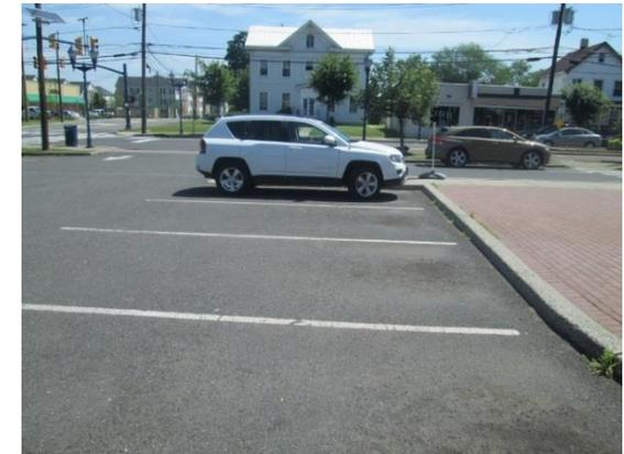
The runoff from the parking area can be captured if the parking spaces were converted to pervious pavement. The building has disconnected downspouts which can be redirected into downspout planter boxes to treat the runoff from the roof. A preliminary soil assessment suggests that the existing soils have suitable drainage characteristics for green infrastructure.
