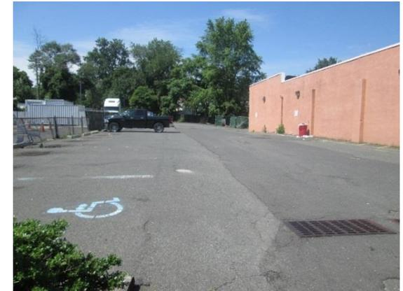
The parking lots drain through a series of catch basins. The building has connected downspouts which can be disconnected, and pervious pavement can be used in the parking lot to capture both road and roof stormwater runoff. A preliminary soil assessment suggests that the existing soils have suitable drainage characteristics for green infrastructure.
