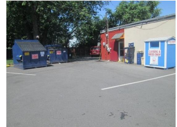
The paved parking lot drains toward the street. Pervious pavement could be utilized in the parking spaces to allow infiltration of runoff before it reaches the street's drainage system. A preliminary soil assessment suggests that the existing soils have suitable drainage characteristics for green infrastructure.
