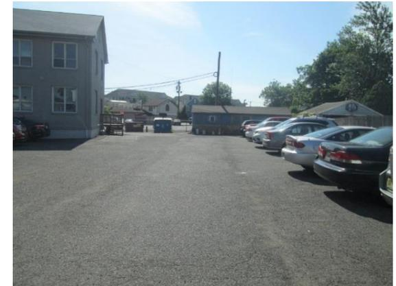
The building's parking lot slopes toward the road. Pervious pavement can be installed in the parking spaces near the building to capture this runoff. In front of the building the turf grass area can be converted into a bioretention system, and downspouts can be disconnected and redirected to allow roof runoff to infiltrate. A preliminary soil assessment suggests that the existing soils have suitable drainage characteristics for green infrastructure.
